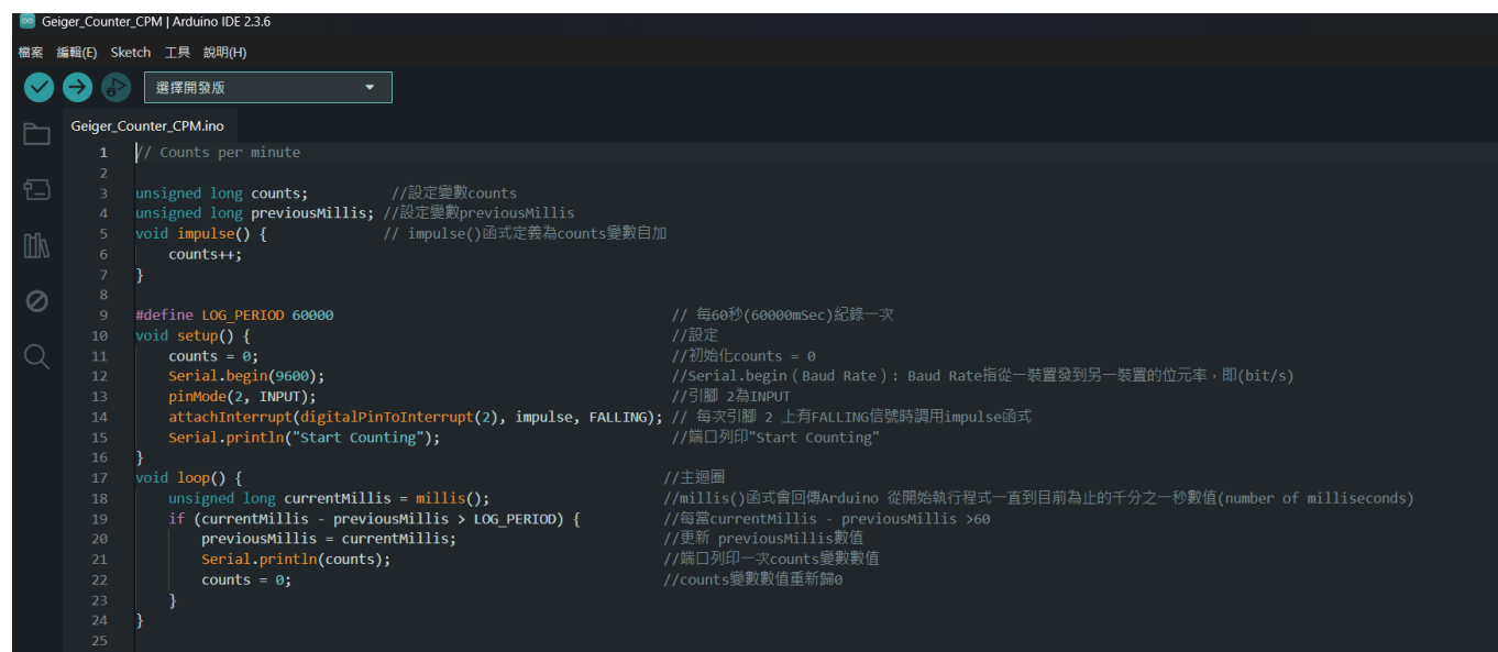
Figure 2. The user interface of the Arduino IDE and the basic code of this experiment. The program code was configured to transmit cumulative counts every 60 seconds.
